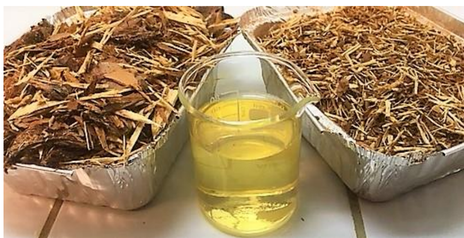
Figure 4-5. Photograph of the original (left) and milled (right) pine bark sample, as well as extract sample from one experiment from case 1.
