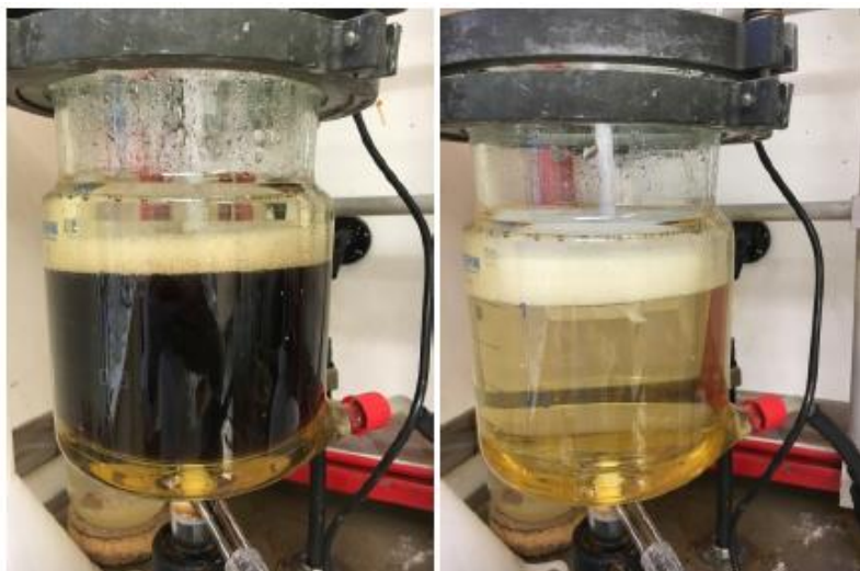
Figure 4-1: Foam solidity test. To the left: Bark extract. To the right: Spuma.
