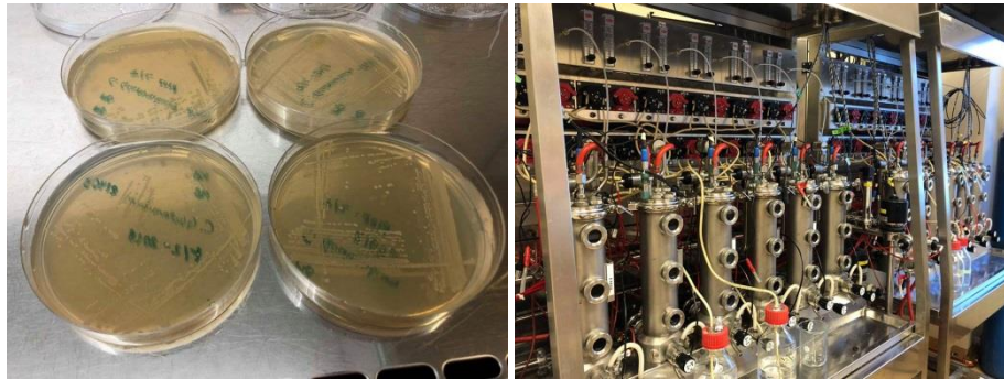
Figure 2-4. To the left is a picture of Corynebacterium glutamicum and Bacillus subtilis strains streaked on agar plates. Right: the 1 litre multiple bioreactor system used in microorganism culture and fermentation trials at the facilities of RISE Processum AB in Örnsköldsvik.
