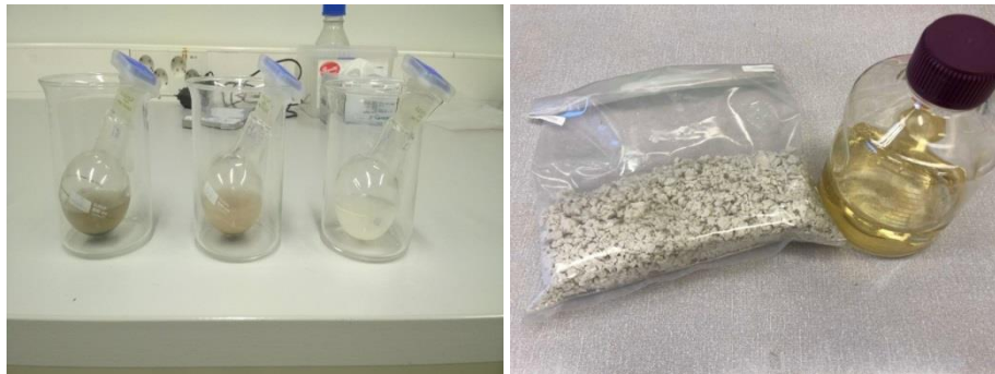
Figure 2-3. Left: picture of three of the four types of fibre sludge provided by the industrial partners UPM Kymmene Pietarsaari, SCA Obbola, Domsjö Fabriker and Metsä Board Husum. Right: Fibre sludge in dry solid form and hydrolysate after enzymatic hydrolysis.
