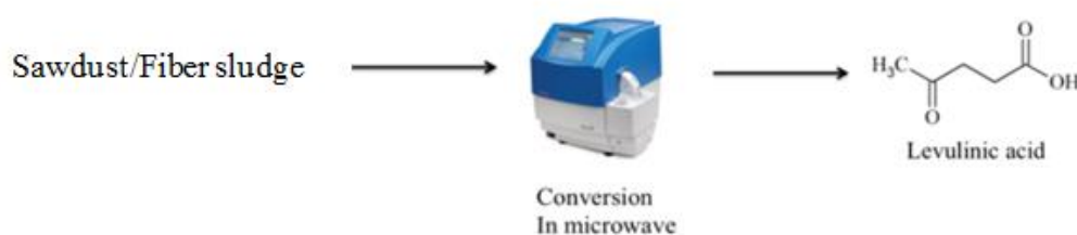
Figure 1-4: 1-step process conversion of sawdust and fiber sludge into levulinic acid.
